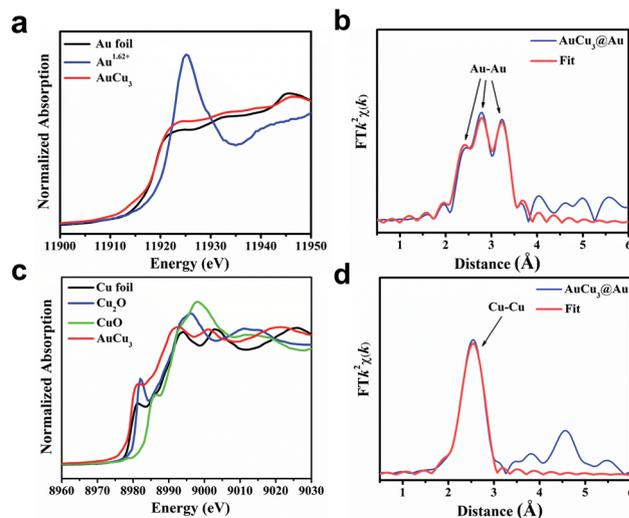
Fig. 3 X-ray absorption fine structure spectra of AuCu<sub>3</sub>@Au. (a) XANES profiles at the Au L<sub>3</sub>-edge. (b) EXAFS spectra at the Au L<sub>3</sub>-edge. (c) XANES profiles at the Cu K-edge. (d) EXAFS spectra at the Cu K-edge.
