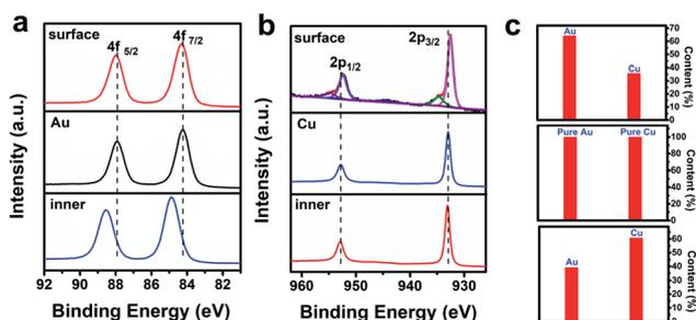
Fig. 2 High-resolution XPS spectra of surface nanoporous AuCu<sub>3</sub>@Au, pure Au, pure Cu and inner nanoporous AuCu<sub>3</sub>@Au. (a) Au 4f region, (b) Cu 2p region, and (c) Au and Cu content diagram.
