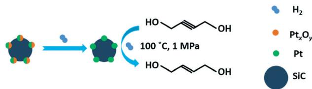
Scheme 1 Schematic presentation on structural evolution of Pt/SiC catalyst for selective hydrogenation of 2-butyne-1,4-diol reaction (BYD) to 2-butene-1,4-diol (BED).
